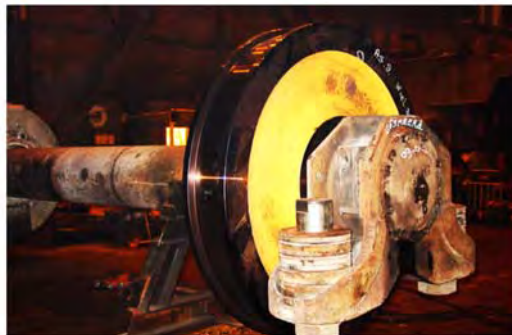
Wheels Ø 1.200 mm on a drive axle of a steel ladle transfer car
